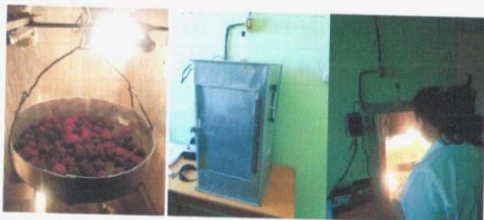
Pic.3. Drying berries under infrared heating in laboratory dryer
